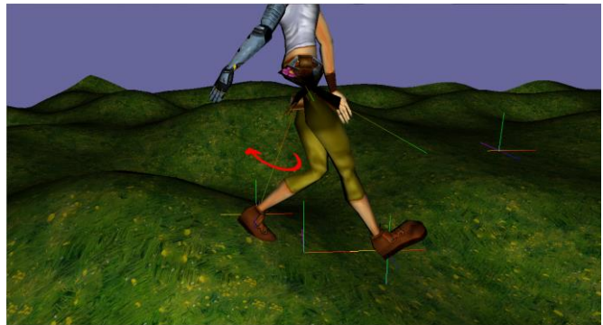
Fig. 9. Using formulas presented in [3], the final rotation uses the axis that preserves the foot location to minimize the angle between initial artist or motion capture data and the position calculated via inverse kinematics to reach a desired foot location. Minimizing using a forward vector for the bone rather than the vector aligning with the thigh produces consistently correct results.
