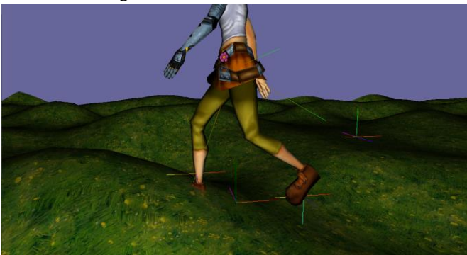
Fig. 4. Original walk animation, adjusted vertically for height of terrain but without any form of inverse kinematics. The right foot clips almost completely into the terrain surface and the left foot is floating far above the ground.
