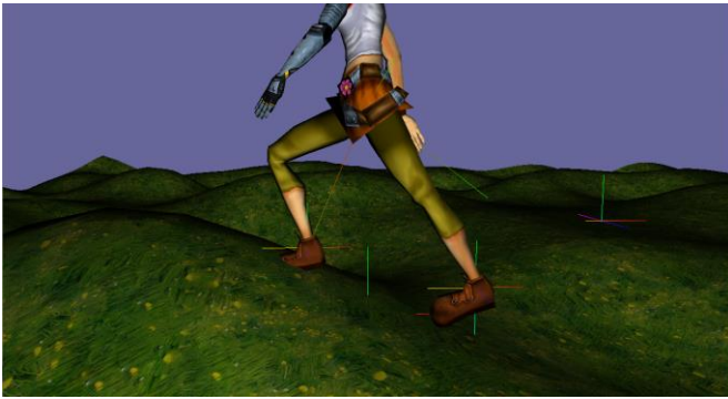
Fig. 10. Final animation, with inverse kinematics placement of feet, looks more realistic than the artist animation alone. Axes near the ankles show the better positions used to place the feet, and vectors extending from the thigh bone (visibly near the hip) show the initial and final positions for the leg, as well as the axis of rotation between the two.
